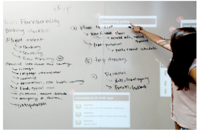
Figure 2. Crowdbord 1.0 (studio interface). A physical whiteboard is augmented with crowd ideators’ comments projected onto the physical board.
