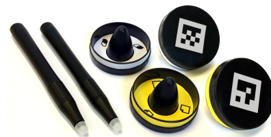
Figure 6. CrowdBoard 2.0 tools: IR-pens for drawing and barcode-based tools for erasing and creating virtual sticky notes.
